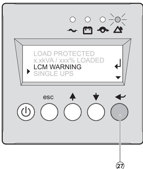
Press the "Enter" button (27) to display LCM warning details.
